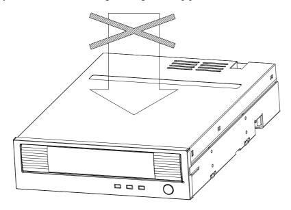
• Use screws of which length inside the drive should be more than 2.5mm and less than 3.5 mm from the drive frame surface.
